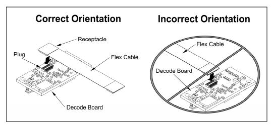
Figure 40. Flex Cable Orientation – Decode Board
